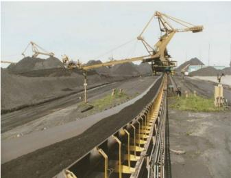
2. tripper belt conveyor is the general band conveyor type finalized in 1990s, Its characteristics were large volume, strong climbing ability and convenient maintenance, etc, It can not only meet the standard of leveling, lifting and decline transportation requirements, but also the convex arcs, concave arc and linear combination transportation methods.
