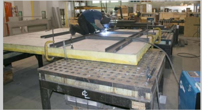
Custom Floor Section Being Fabricated
